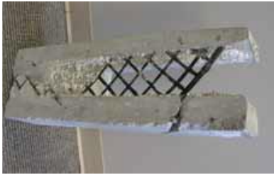
Figure 5.1 Sandwich panels with FRP connectors (a) Tested panel with FRP shear grid (Frankl et al., 2011) (b) Cross section of test panel (Hopkins et al., 2014)
