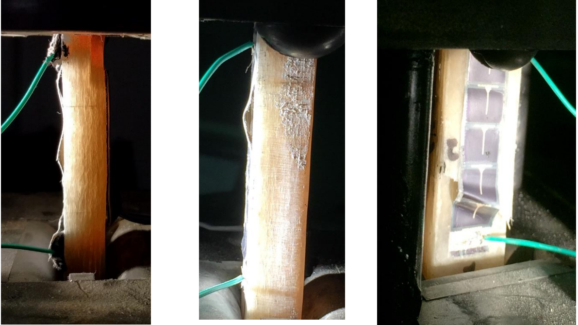
Figure 4.17 Different modes of buckling of amorphous silicon solar subjected to compression loading
