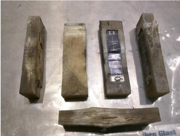
Figure 4.22 A-Si compression samples failure modes
