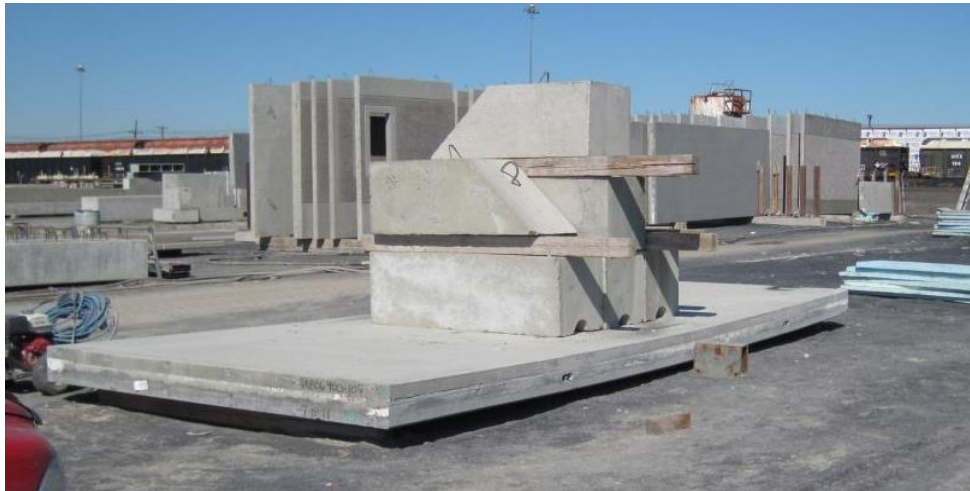
Figure 2.5 Final load placement
