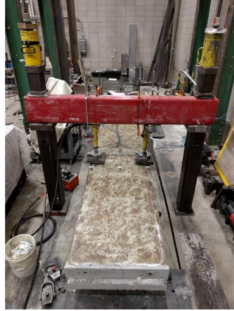
Figure 3.13 PVICS panel under three-point loading
