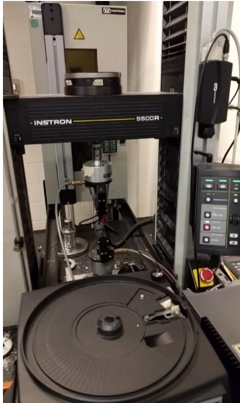
Figure 4.11 Tension setup for perovskite solar cell samples
