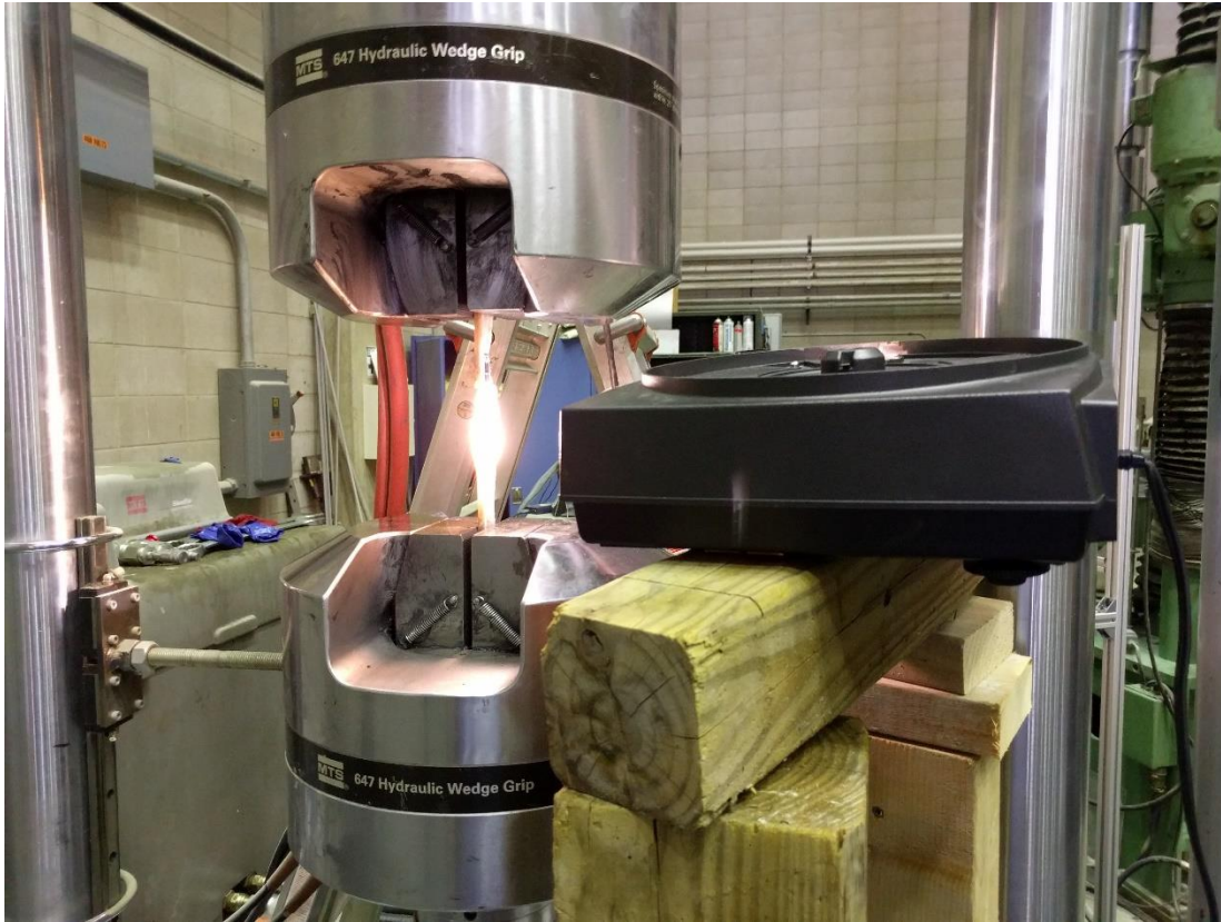
Figure 4.9 Compression test setup under Kodak carsoul projector illumination
